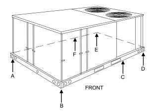
FIGURE 11 - FOUR AND SIX POINT LOADS
